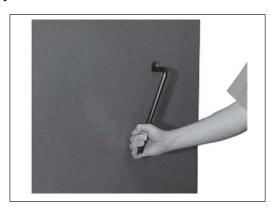
☐ Move the lever of the cleaning system several times before heating up (up and down 5 – 10 times)
